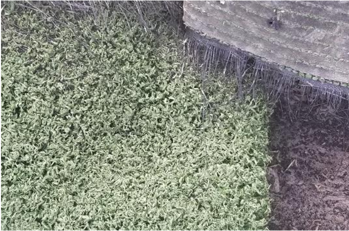
Photo of old field turf showing wear and tear that necessitated replacement
